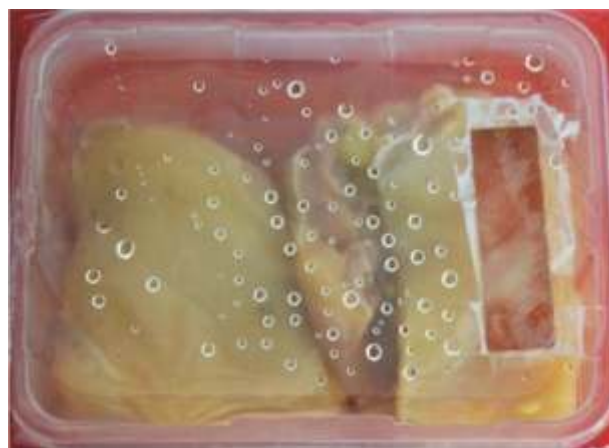
Sticker type sensor shows brownish red while meat quality deteriorates
