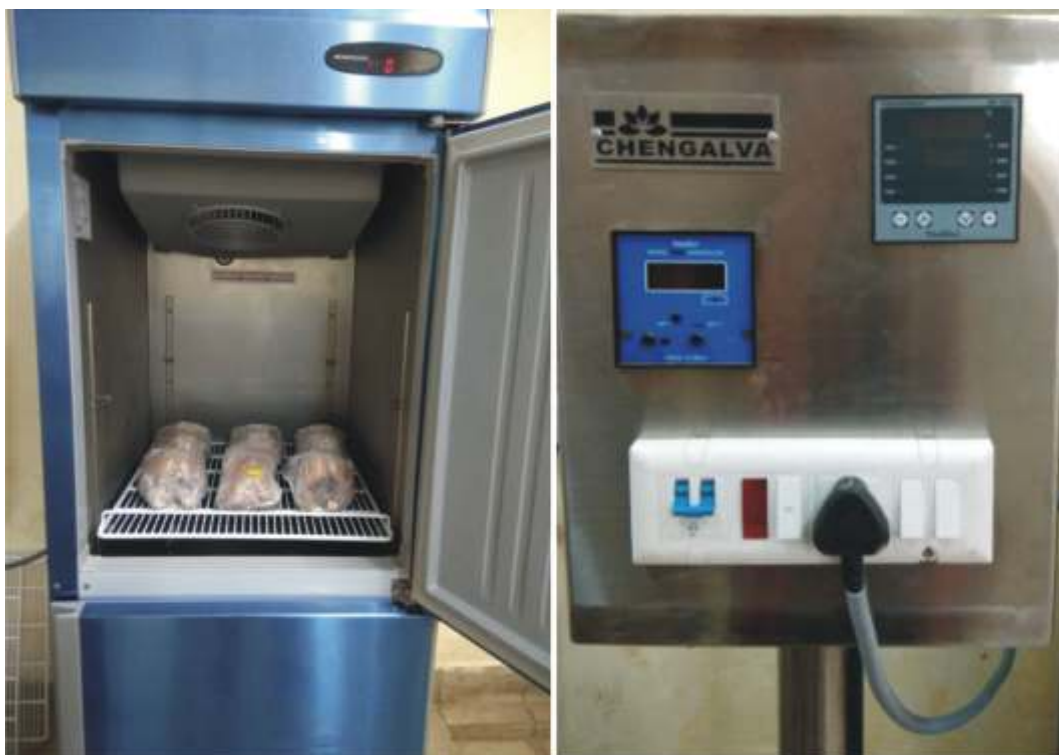
Superchilling cabinet with display unit
