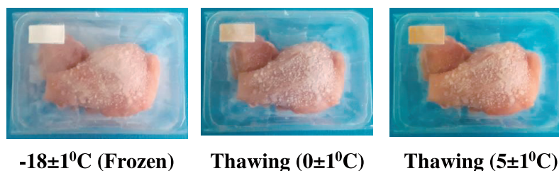
Figure 3 : Images of chicken meat and temperature abuse sensor subjected to different temperature fluctuations during frozen storage
