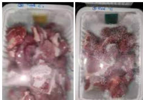
Comparison of oxygen-indicating film colour transition between intact MAP and tampered MAP groups
