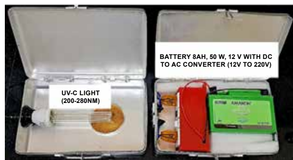
Portable UV Aluminum Cabinet for inactivation of B. anthracis spores in soil
