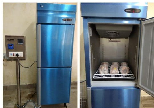
Super-chilling cabinet designed at ICAR-NMRI, Hyderabad
