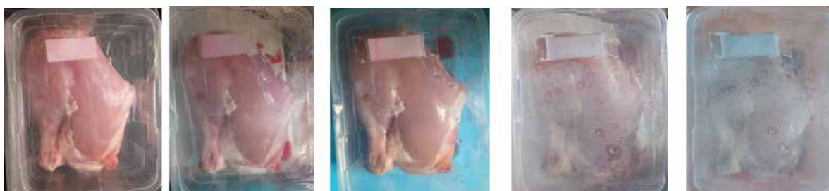
Color change in sticker-type meat freshness sensor (anthocyanin-curcumin-gold nanocomposite) during refrigerator storage (0,3,5,7 & 9 days) of chicken meat
