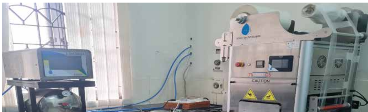
Modified atmosphere packaging machine with gas mixture
