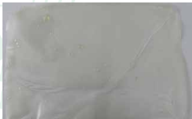
Biodegradable nanocomposite packaging film with sealing property
