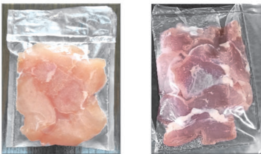
Fig.7. Chicken meat and Pork packaged in biodegradable nanocomposite film
